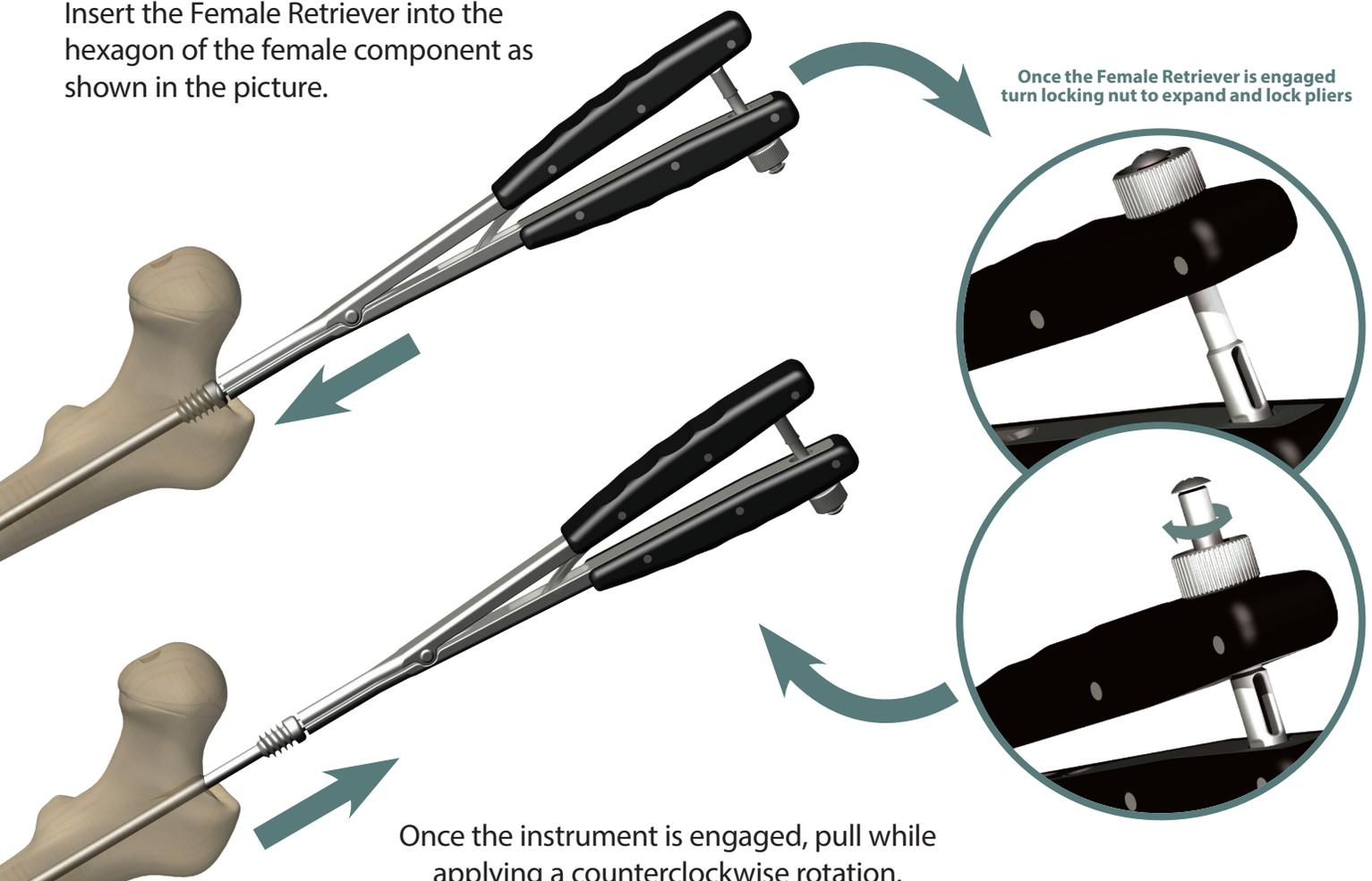
Once the Female Retriever is engaged turn locking nut to expand and lock pliers
