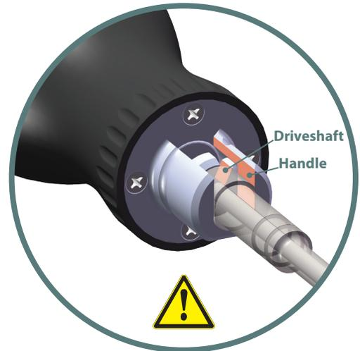
If the driveshaft flats are not parallel to the flat on the handle, the disassembly will not be possible.
