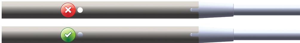
**⚠** Tightening of the Male Retriever handle without the male component inside will result in damage to the shaft and render it unusable. A new Shaft will be necessary since they are single use instruments.
