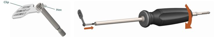
Ensure that the notch of the Cone Shaft is aligned properly with the Hex. If the Clip moves and the Hex falls of the notch, it is important to reassemble it properly before continuing with the next steps.
