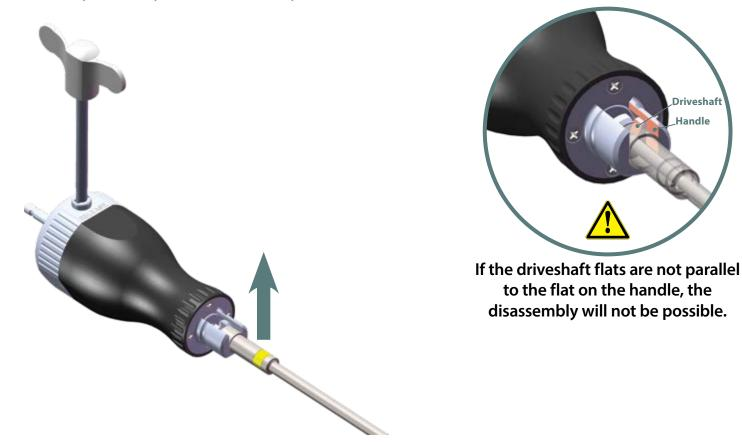
To align the flats, maintain the Release Button depressed with the Release Key, then rotate the Driveshaft clockwise until the flats line-up. The Shaft and Tube assembly can then be pulled upwards.
