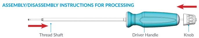
**CAUTION:** If required, use the Cap Driver to unlock the Knob with a counterclockwise rotation.
