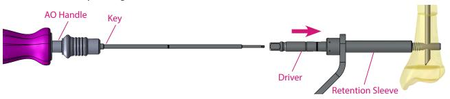
Visually validate that the Bullet window is open using the markings on the instruments.
