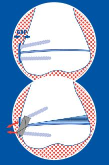
The Hinge Plate continuously conforms to the surface of the bone without stresses or forces producing an unrestrained angular correction around a *true hinge*.
